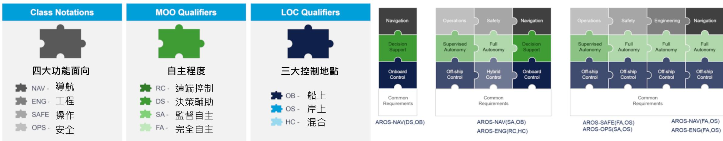
Autonomous and Remotely Operated Ships (AROS) family of class notations
